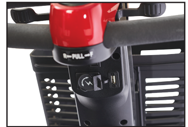
4. USB & Battery Charging Ports conveniently located on the tiller under the control panel.
